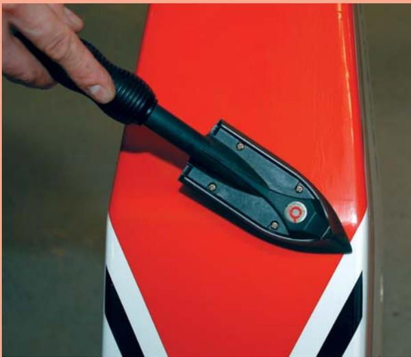
2) Using your covering iron with a soft sock, gently apply pressure and rub in the covering. If any bubbles occur, your iron may be too hot. Reduce heat and work slowly.
