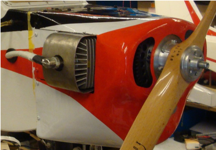
Engine 2) special air extractor lower duct wall in place to extract air over the lower cooling fins using the cylinder jacket air guiding. (no temps taken)
